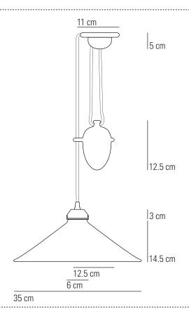
Cable length may be shortened upon installation. This will reduce both maximum & minimum dropand reduce the range of movement.
