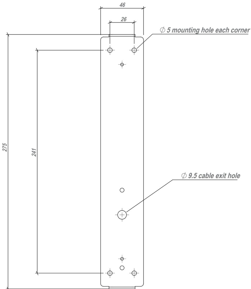
Backplates can be rotated 180 degrees- to allow cable exit to be positioned at top if required.
